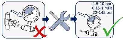
Figure 7. Low pressure restart function
